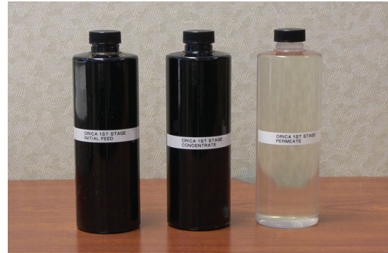
Figure 1: Initial Feed (Left) Concentrate (Middle) Permeate (Right)
