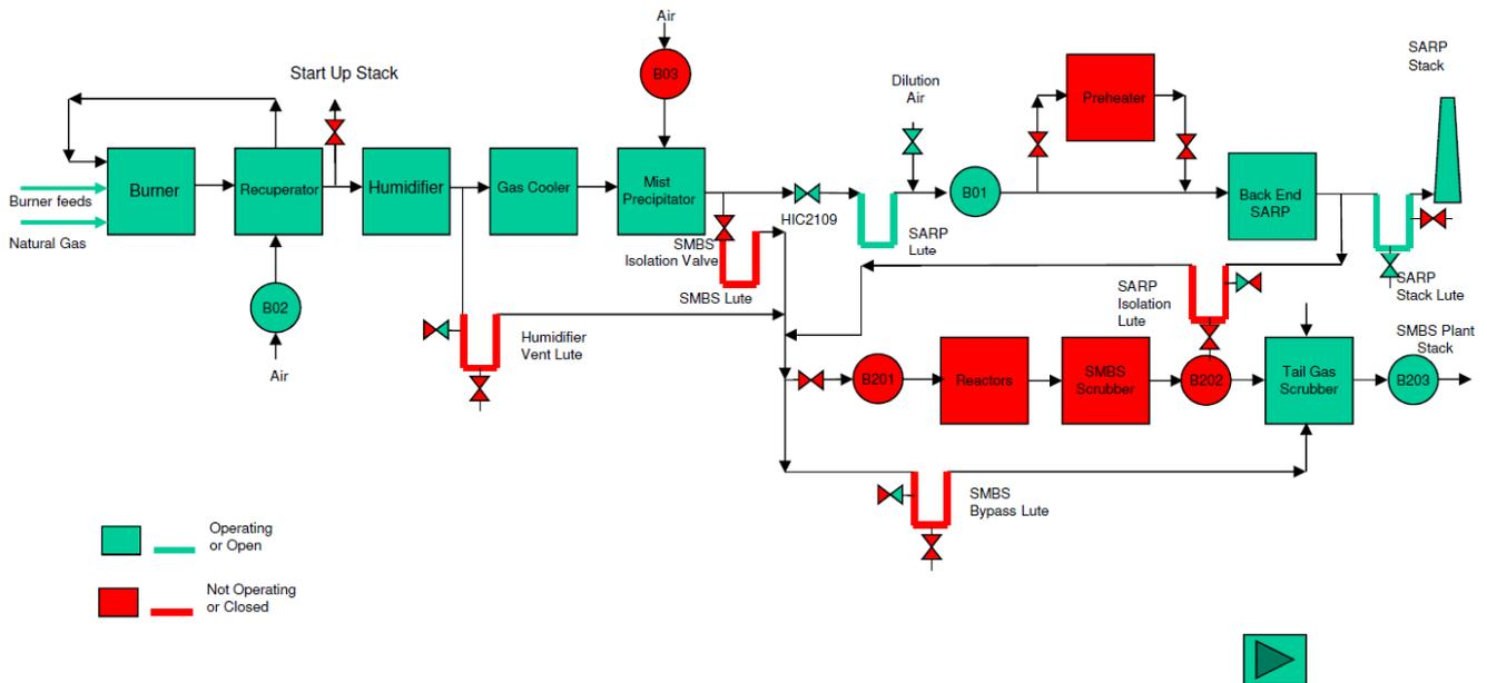
SARP: Emergency trip system in operation diagram
